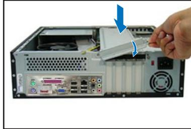
2. Match and insert the hooks of the cover to the elongated holes on the side of the chassis. All eight hooks (four hooks on both sides) of the cover must properly fit the designated holes.
