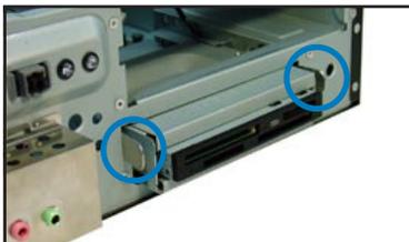
3. Press the card reader lock inwards (A), then slightly pull the card reader assembly outward (B) until the USB cable and plug is exposed.
