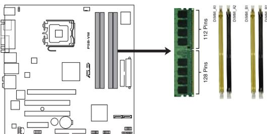
**P5B-VM 240-pin DDR2 DIMM socket**
