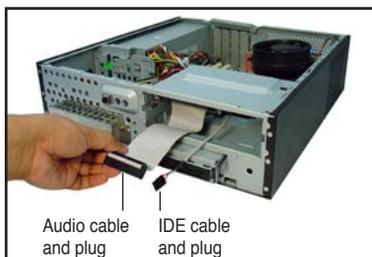
5. Connect the IDE cable to the IDE interface at the back of the drive. Match the red stripe on the cable with Pin 1 on the IDE interface.
