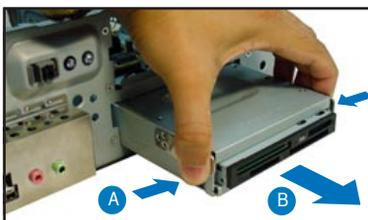
4. Disconnect the USB cable and plug from the card reader assembly, then set the card reader assembly aside.
