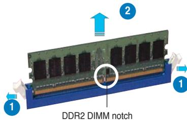
2. Remove the DIMM from the socket.
