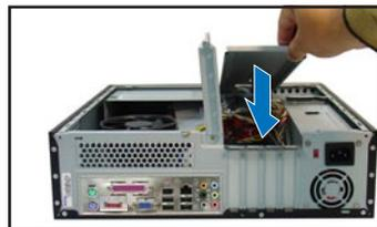
6. Replace the expansion card lock to secure the card to the chassis.
