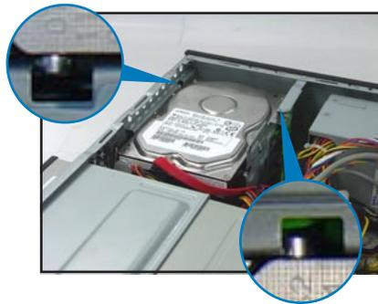
6. When the HDD screws align with the screw rails, push the drive carefully until it is completely flushed on the bay.
