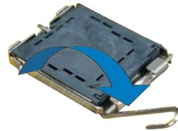
4. Lift the load plate with your thumb and forefinger to a 100° angle (A), then push the PnP cap from the load plate window to remove (B).
