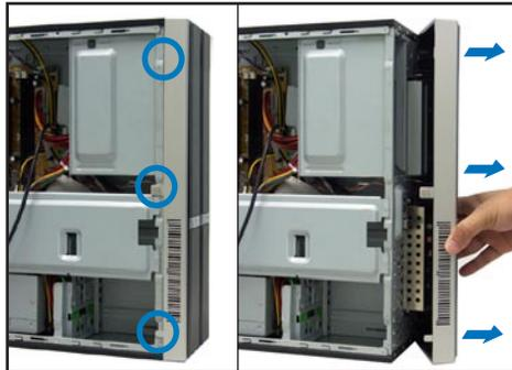
4. Swing the left edge of the front panel assembly outward.
