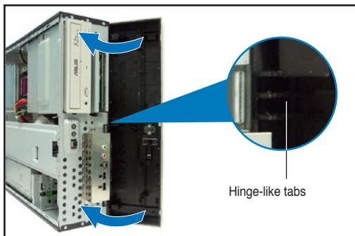
2. Swing the left edge of the front panel inward, then attach the front panel assembly hooks to the chassis until they snap in place.
