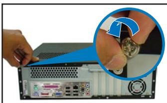
3. Slightly pull the cover toward the rear panel until the cover hooks disengages from the chassis holes.
