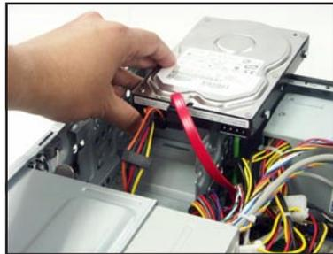
5. Place the HDD on the tray. Make sure that the HDD screws are aligned with the screw holes and rails.
