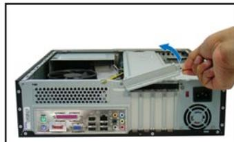
2. Remove the chassis support bracket.
